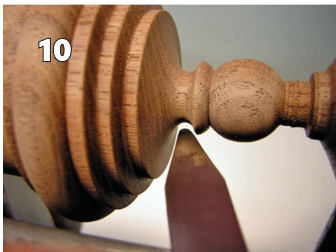
This is one of the rare times you will see me scraping a spindle turning.
