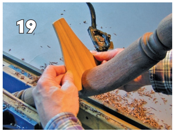
Frequent checking with a circular template keeps everything smooth.
