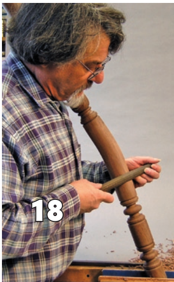
← A double-cut file further refines the surface.
