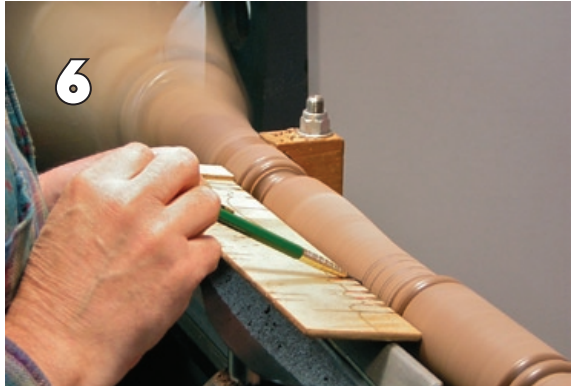
The marking jig has notches to locate the pencil, and marks are drawn while the work is rotating.
