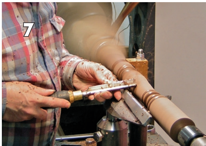
A spindle roughing gouge shapes the work quickly.
