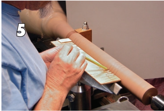
The marking jig has notches to locate the pencil, and marks are drawn while the work is rotating.
