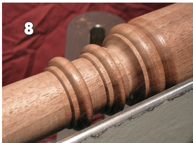
This is the appearance of the work before sanding. Sharp tools + careful work = less sanding.
